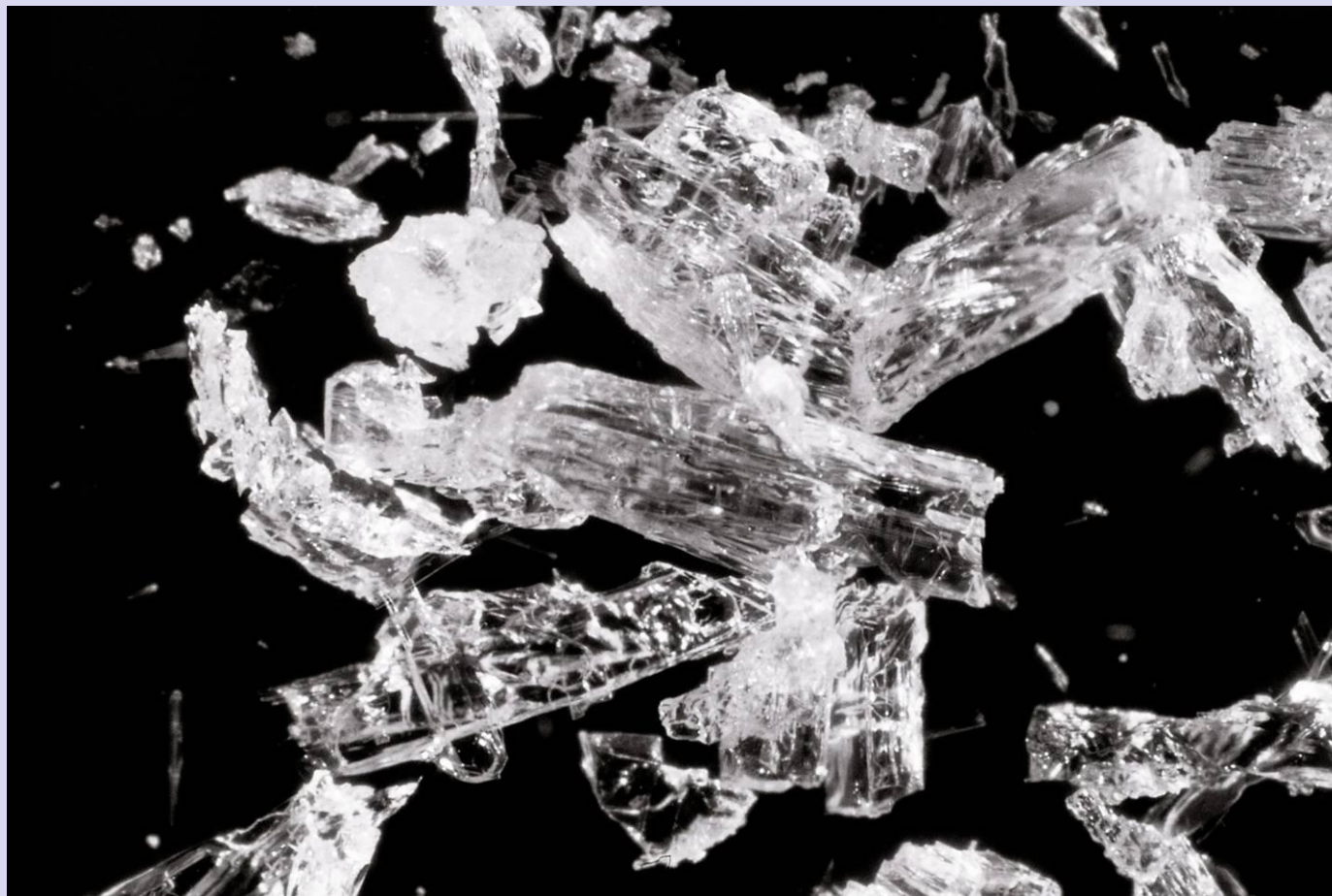
Benzoic acid crystals batch experiment, average size \sim 1500 \mu\text{m}
