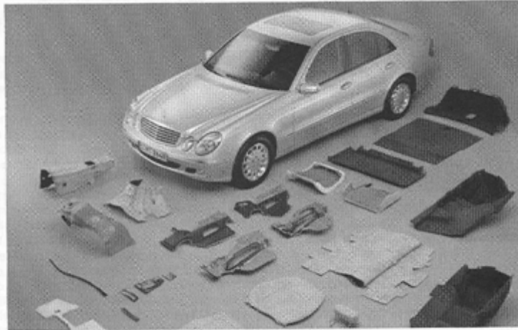
Figure 2.4 Flax, hemp, sisal, wool and other natural fibers are used to make interior Mercedes-Benz E-Class components. (www.daimlerchrysler.com)
