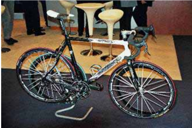
Flax-Carbon hybrid bike (JEC 2007) (prepreg technology)
